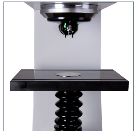
The optional 450mm x 350mm large testing table with T-slots can be used for large and heavy workpieces.
