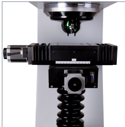
The NEXUS 7501 can be equipped with manual and motorized X-Y stages. Above picture shows optional 250Kgf motorized X-Y stage
